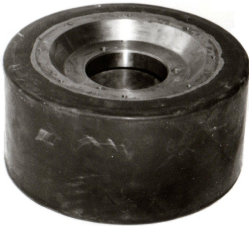
Fig. 1. Sample ring transducer
